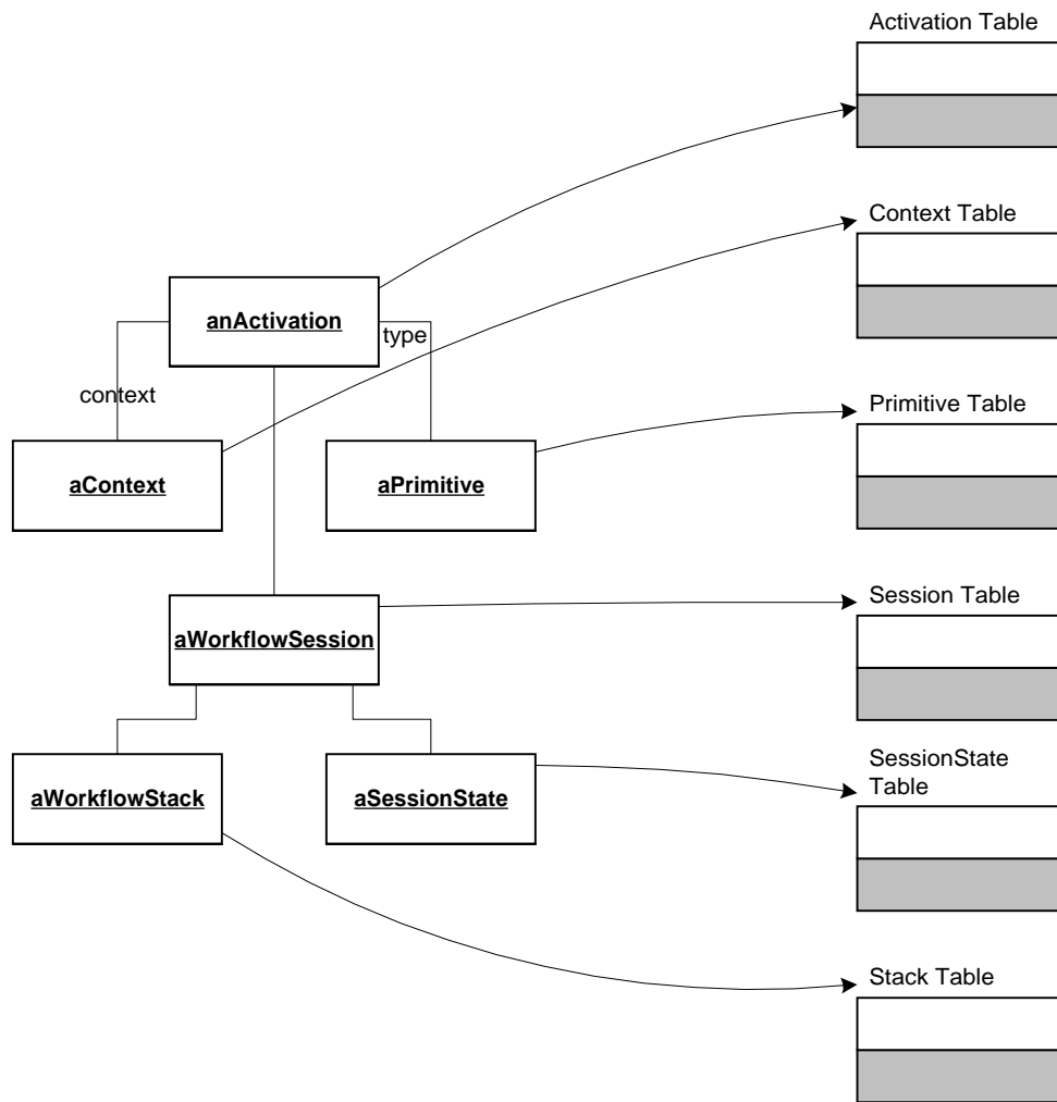
Figure 5.17: Object-to-relational mapping when each class maps into a single table.
